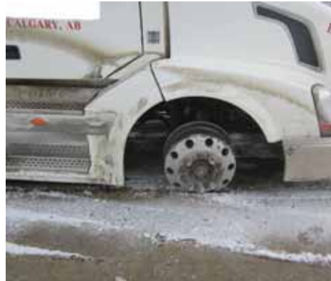
Lost front wheel. Photo by Ofc. Kevin Chaput, Watson Lake Scale, Yukon.
