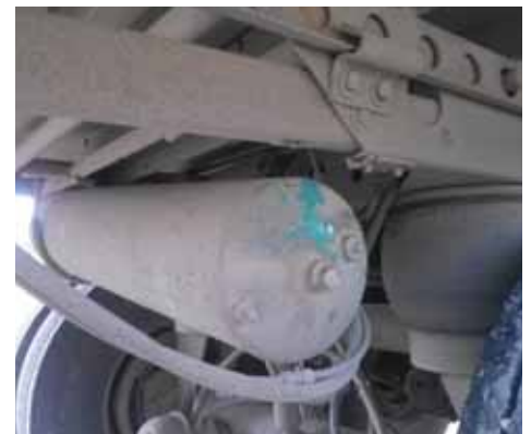
Loose air tank on trailer. Photo by Ofc. Michael Kasprzak, Whitehorse Weigh Station, Yukon.
