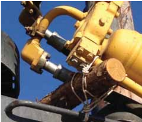
Inadequately secured load. Photo by Ofc. Carol Bates, Whitehorse Weigh Station, Yukon.
