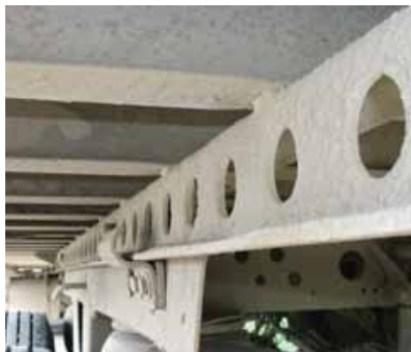
Disengaged slider-guide/hold-down bracket. Photo by Ofc. Michael Kasprzak, Whitehorse Weigh Station, Yukon.
