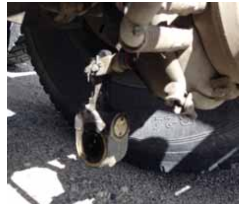
Bad slack adjuster/pushrod. Photo by Ofc. Sheldon Barteaux, Whitehorse Weigh Station, Yukon.
