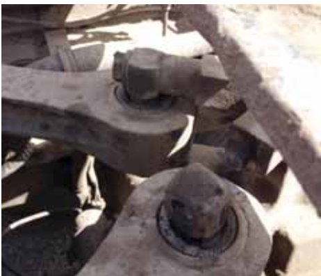
Suspension tracking component gone awry. Photo by Ofc. Sheldon Barteaux, Whitehorse Weigh Station, Yukon.
