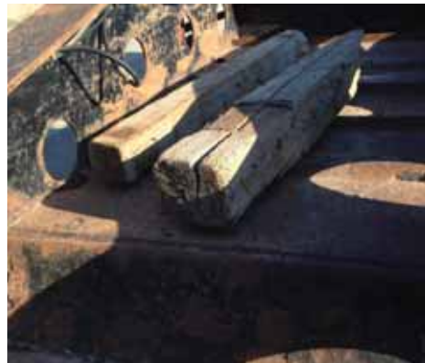
Inadequately secured dunnage. Photo by Ofc. Carol Bates, Whitehorse Weigh Station, Yukon.
