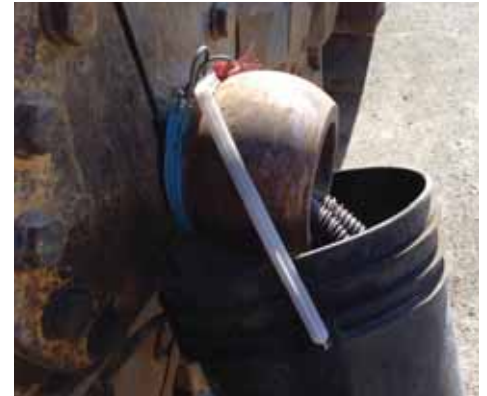
Inadequately secured cargo. Bucket tied to side of a Kubota dozer track. Photo by Ofc. Carol Bates, Whitehorse Weigh Station, Yukon.
