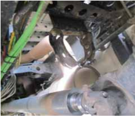
Driveline worn through steady bearing. Photo by Ofc. Kevin Chaput, Watson Lake Scale, Yukon.
